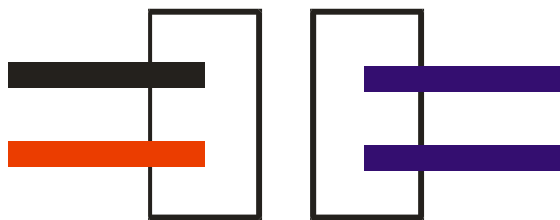
Figure 13-4: Battery Connector Terminals are shaped to connect in the correct orientation. Power connector (black and red) is the left connector, temperature monitor are blue connectors to the right.
