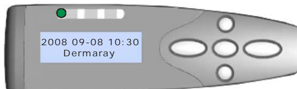
Figure 6-7: Dermalary Welcome Screen is shown on subsequent WAKE commands after completion of the Setp Wizard. The screen displays the YEAR – DATE – TIME and a logo.
