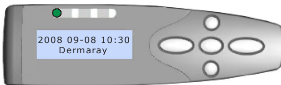
Figure 5: Dermaray Welcome Screen is shown on subsequent WAKE commands after completion of the Setup Wizard. The screen displays the YEAR – DATE – TIME and a logo.
