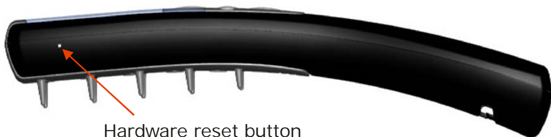
Figure 10-11: Hardware reset button. Once pressed, the LCD display will flash and beep.
