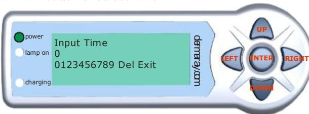
After entering the Manual Treatment Time either 1.Complete the setting and begin the treatment, 2.Discard & Exit or 3.Cancel and return to the Input TIME screen. Once started a treatment surface must then be detected before the lamp will activate.
