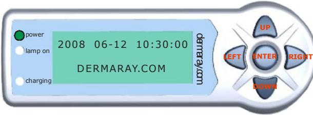
Press and hold the DOWN button for 3 seconds to manually activate the UV lamps, with proximity detection and with a user defined countdown timer (shut off will occur once timer has expired).
