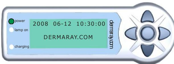
**To turn Off UV lamp (enter sleep mode) at any time and at most menus to turn off** Dermaray UV lamp, PRESS and HOLD the ENTER button for 3 seconds. This will turn the unit OFF and is called SLEEP mode.
