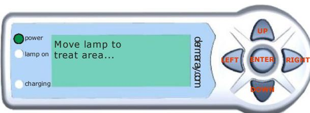
Once a surface is detected the UV lamp will turn on and the treatment will be administered. The RED LED will also be activated to indicate the UV lamp system is active.
