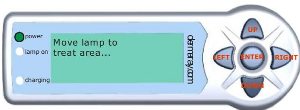
Once a surface is detected the lamp will turn on and the treatment will be administered. The RED LED will also be activated to indicate the UV lamp is active. The timer will display with the time REMAINING for this treatment session. A session can be STOPPED, PAUSED or SKIPPED by pressing ENTER during the session
