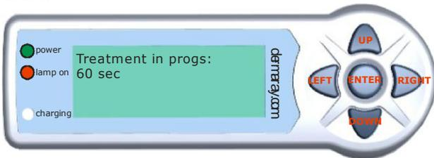
**NOTE:** This is a timer that decreases from the specified time limit. In this mode, the lamp will remain on until automatically de-activated when the timer reaches zero or manually stopped by pressing ENTER and selecting STOP, or when proximity detection pauses the countdown.
