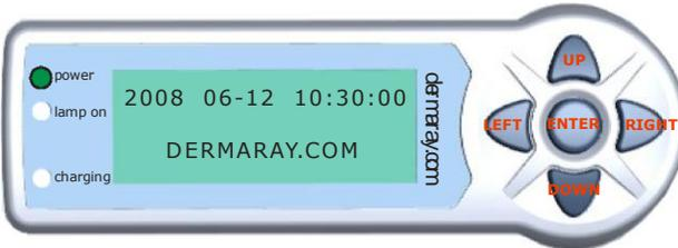
Press and hold the UP button for 3 seconds to manually activate the lamp. Dermaray<sup>□</sup> - UV lamp will start counting how long it is activated for. Once started a treatment surface must then be detected before the lamp will activate. This mode must be stopped manually.
